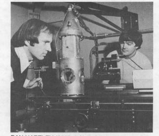
DAN HARTLEY (6000, left) and Pete Witze (DMTS, 8362) in 1975 setting up laser Doppler velocimeter on high pressure flame facility during early days of Sandia Livermore's combustion research.
